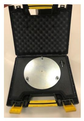
Base plate can be used to monitor vibrations on carpet or wooden floors. The SWARM can be mounted on the Base plate with one bolt.
